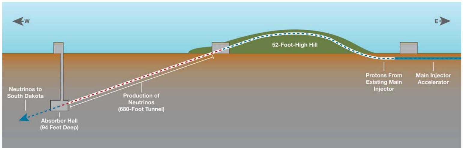
Fermilab plans to use its Main Injector accelerator to make neutrinos and send them through the earth to the LBNE particle detector in South Dakota. The project would require the construction of three buildings, a 52-foot-high hill made of compacted soil and a 680-foot-long tunnel on the Fermilab site.
