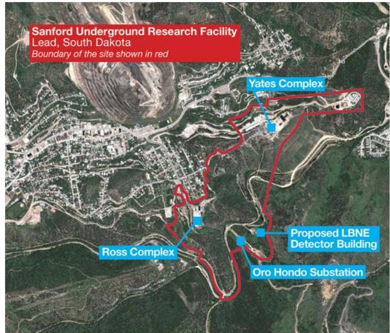
A new building, to be located east of the Oro Hondo substation on the Sanford Lab site, would house the particle detector of the proposed Long-Baseline Neutrino Experiment.
