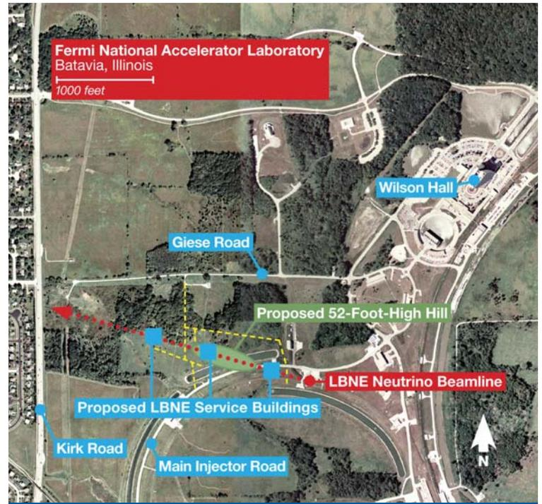
The LBNE neutrino beamline at Fermilab would be located on the western part of the Fermilab site, near Giese and Kirk Road. The locations of the three planned service buildings are marked with blue squares and the footprint of the planned, 52-foot-high hill is marked in green. Planned access roads are marked in yellow. Kirk Road runs along the western boundary of the Fermilab site.
