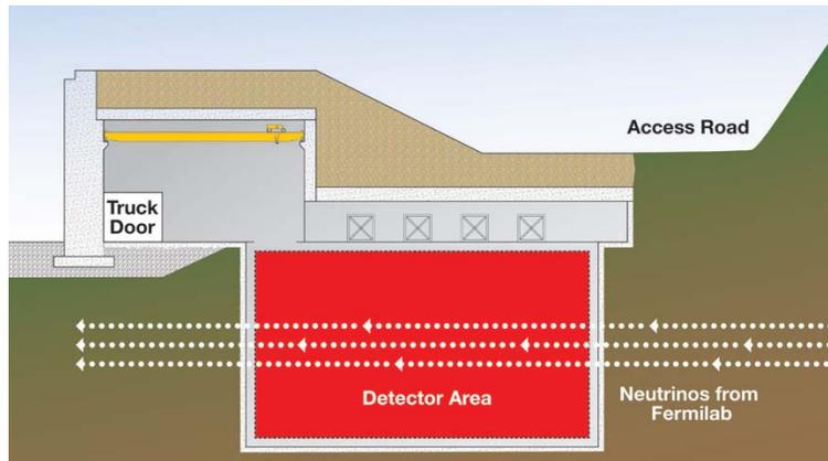
The LBNE detector building would have a basement that would be about 60 feet deep and 100 feet long, to be excavated in surface rock on the Sanford Lab site. A hall on the first floor of the building would house equipment needed to construct and operate the detector. The neutrinos from Fermilab would travel straight through rock and enter the detector from the east. If additional resources become available, scientists would build the particle detector deeper underground.
